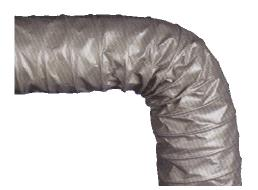
The Model TD8 is an economical air ventilation, fume removal flame retardant hose with vinyl coated woven fiberglass cover permanently bonded to a PVC coated spring steel wire helix. This hose meets UL 181 class flammability ratings and NFPA 90A-90B fire code. It is ideal for low volume air transfer and applications include dry cleaning equipment, air intake and exhaust ducts, heating and cooling systems, dust, and many others.
